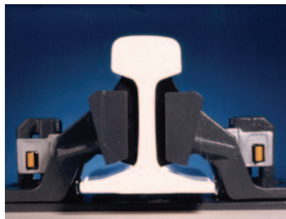
Vanguard resilient rail support. The resilience acts on the web giving low vertical stiffness with high lateral stability (Source: Pandrol Ltd, UK)
