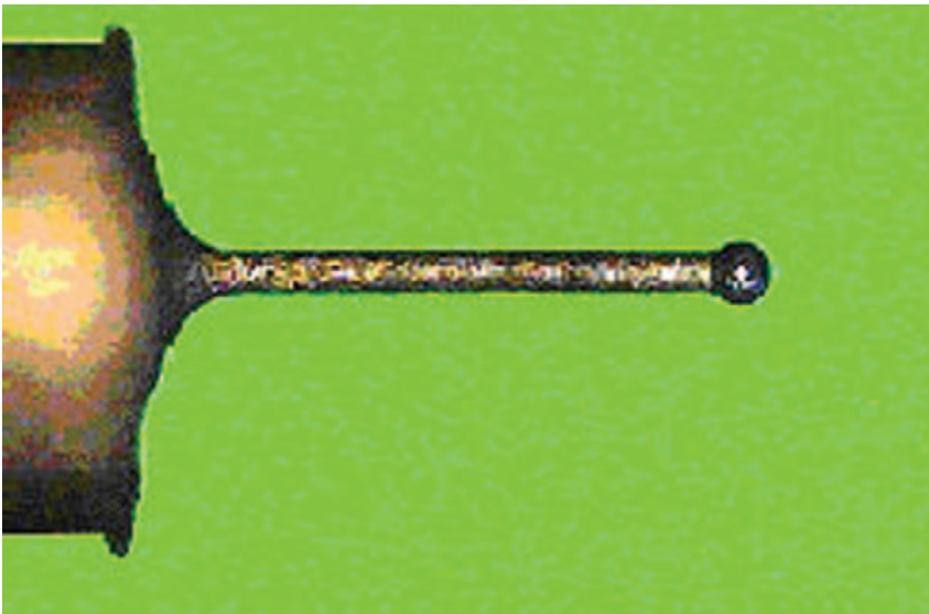
Micro-manufacturing – A micro-turned 'micro co-ordinate measuring machine' (CMM) stylus. Researchers will investigate how to manufacture these devices using a femtosecond laser.
