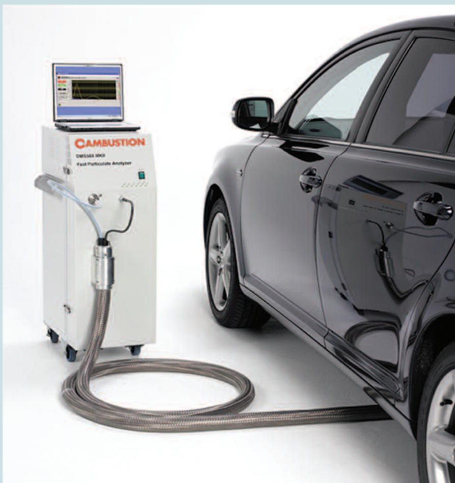
Cambustion's fast response particle analyser is used in the development of cleaner engines
